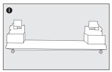
Remove the top spine cover and place the spine on a level surface, with the bulb holders facing upwards.
