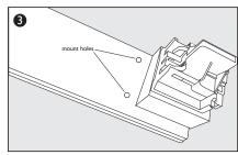
Place the part built shade onto the spine lining up the mounting holes. The bulb holders should be coming through the cutouts in the shade.
