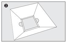
Using 12 of the shorter bolts, nuts and washers, assemble the 4 side panels together, ensuring that the 2 panels with cutouts are opposite each other.
