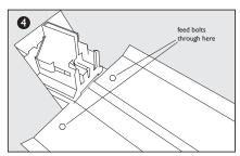
Next, line up the space bar with the mounting holes of the spine and shade, and then do the same with the top diffuser plate. Pass one of the long bolts through the top plate, spacer bar, shade and then spine (in that order). Secure the bolt from inside the spine with a nut and washer. Do this with all 4 mounting points on the spine.
