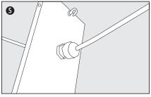
Loosen the gland lock nut and feed your ballasts cable through the gland.
