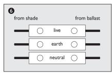
Next, wire your ballast into your shade ensuring that both lives, both neutrals, and both earths are securely connected into the correct place on the connector block. With no stripped cable showing once the wires
